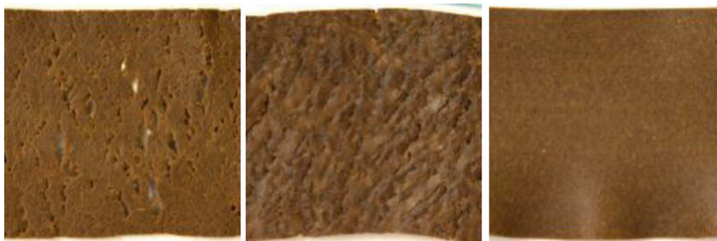
Figure 3. Films extruded from Material C with different die temperatures and pressures: 125°C_3.6 MPa (left); 125°C_5.2 MPa (middle), and 130°C_5.2 MPa (right). [Color figure can be viewed in the online issue, which is available at wileyonlinelibrary.com .]
