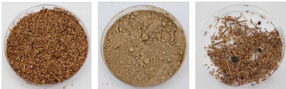
Figure 1. Crambe meal before (left) and after ball milling for 24 h (middle) and the fraction excluded by sieving (right). [Color figure can be viewed in the online issue, which is available at wileyonlinelibrary.com .]
