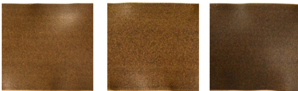
Figure 4. Material D extruded at 125°C_20 rpm (left) and 130°C_20 rpm (middle), and Material E extruded at 125°C_30 rpm (right). [Color figure can be viewed in the online issue, which is available at wileyonlinelibrary.com .]
